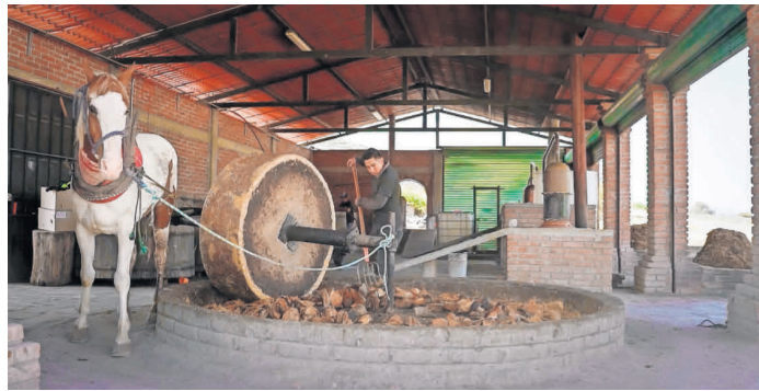
Roasted agave hearts are crushed to extract juice for fermentation. Courtesy of Chulele Mezcal
